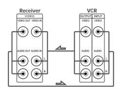
V Use the function buttons (TV/LD, CD, MD/TAPE etc) to select the VIDEO AUDIO OUT signal. You can record this audio signal by connecting a recording component such as a cassette deck (to the VIDEO AUDIO OUT jack).
